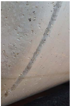
Above: Pitting caused by galvanic corrosion.
