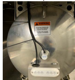
Below: Hull Shield test transducer on pontoon.
