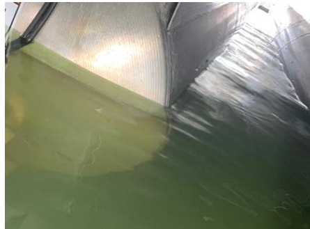
Day 14 Result - Pontoon with Hull Shield HS75
